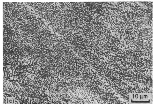
Figure 2 Microstructures of chips of as-cast bars of (a) steel 1A; (b) 2A; (c) 3A. Cutting speed, 66 m min -1 .
