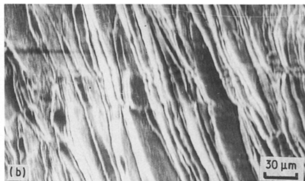
Figure 5 SEM micrographs of the undersides of chips (a) steel 1A; (b) 2A; (c) 3A.
